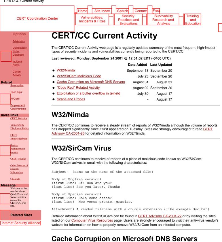
The CERT/CC has received reports from sites experiencing DNS cache corruption on systems running Microsoft DNS Server. The default configuration of this software allows for data from malicious or incorrectly configured DNS servers to be cached and supplied to client computers using that cache to resolve DNS information.
